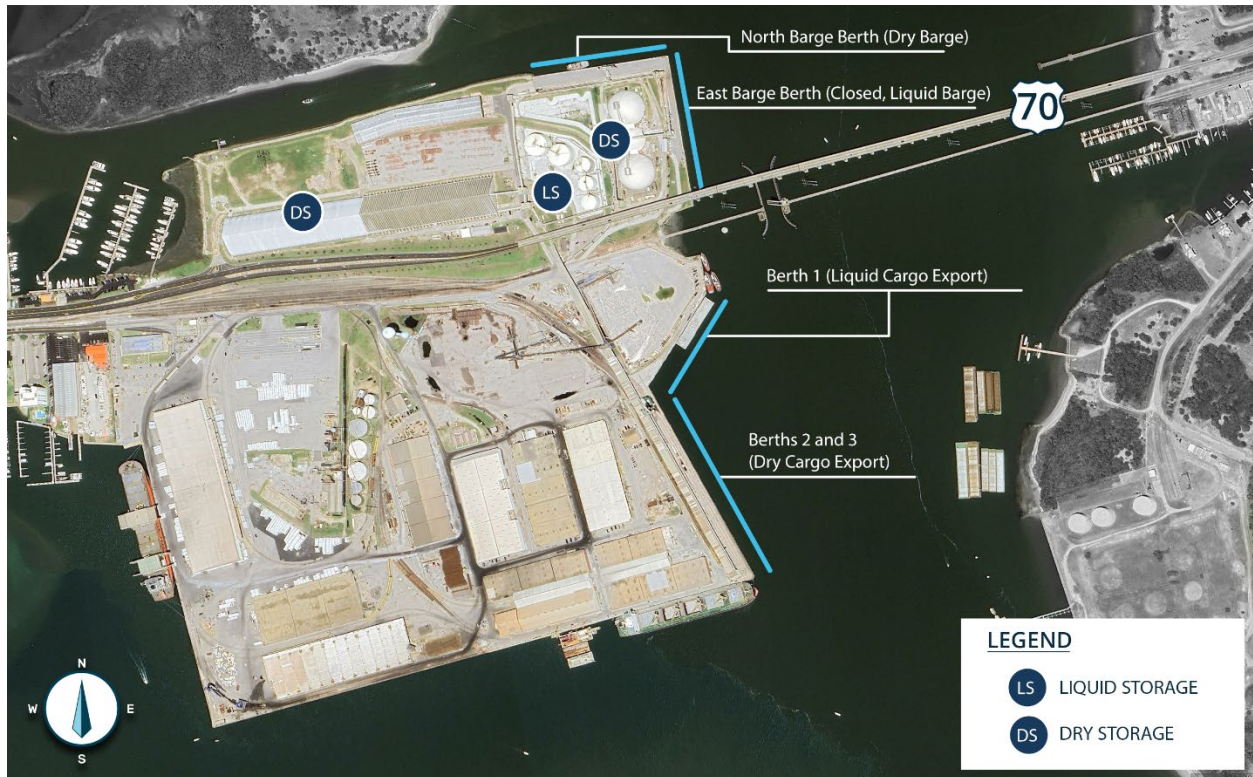
Figure 1. Without the Project, barges must navigate the narrow passage beneath the Newport River Bridge (US 70) to unload at Berth 1.
